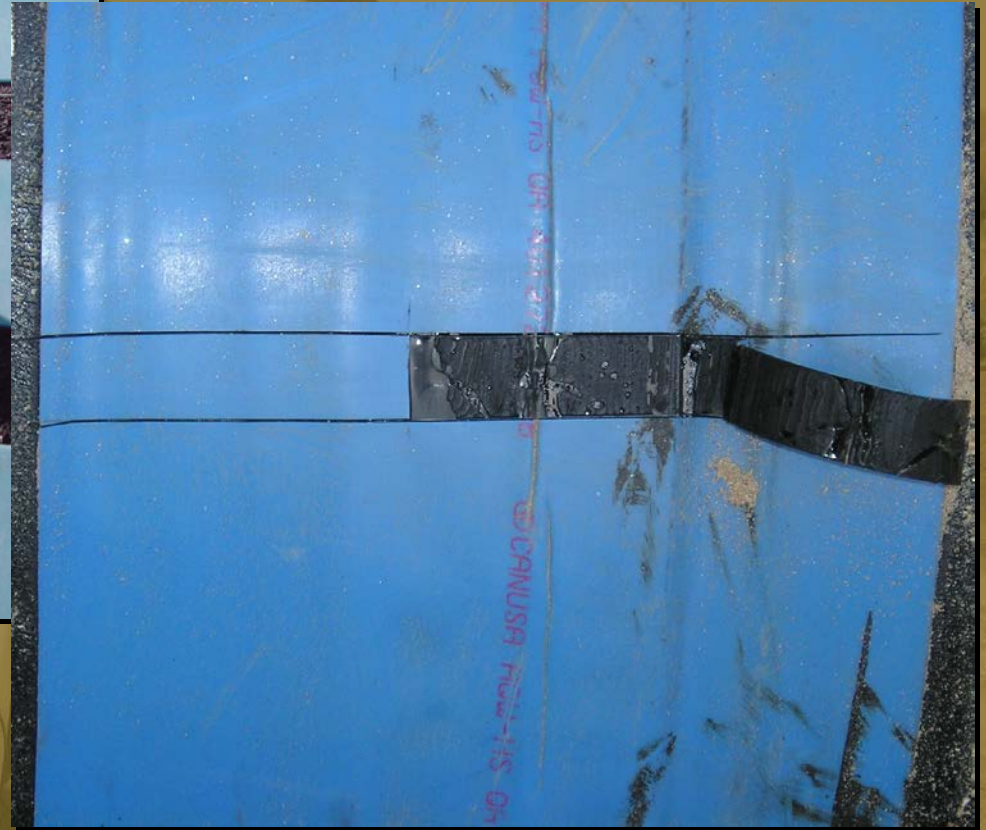
PE backing visibly affected but adhesion good
